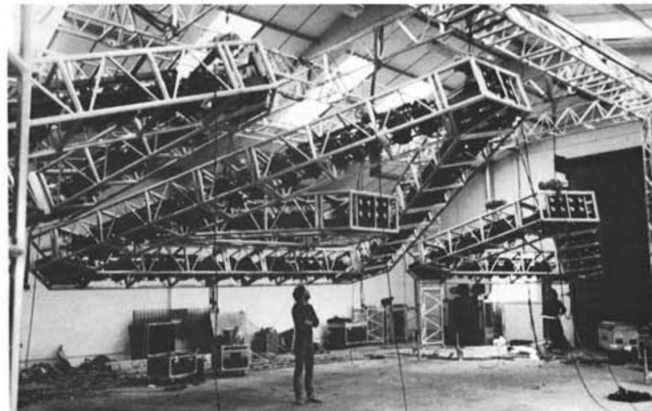
The elaborate and pioneering rig for Iron Maiden during construction in a rented warehouse in 1983. The rig had its own ground support gantry, just visible in this picture.
